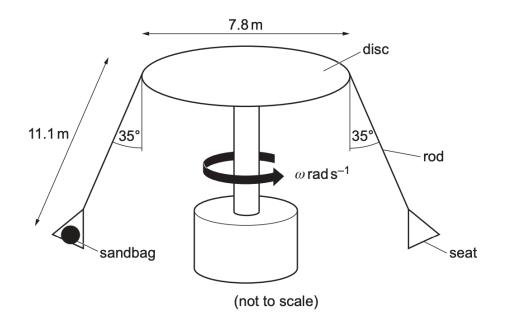
Assuming uniform circular motion, what is the angular speed  $\omega$  of the system?
