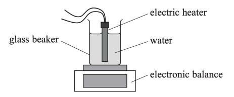
The heater supplies a constant power of 120 W for 5.0 min and the balance records a mass loss of 34 g. What experimental value of the specific latent heat L of water is obtained?
